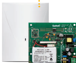
ABAX 2 DEVICE SIGNAL RETRANSMITTER
